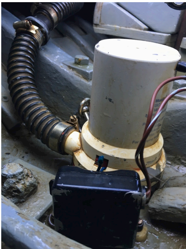
Bilge pump and separate solid state 'float' switch showing inline non return valve
