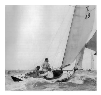
A local naval architect, Sidney Graham, was commissioned to lift a set of lines of an existing boat, then make a number of changes. The "new" boat was lengthened a little and the draught reduced. Most significantly the centerboard was replaced with a fixed keel. At the same time, Charles Nicholson developed a new rig for the boat – Bermudan rather than Gaff, with a small jib and large main set on a boom that overhung the transom.
